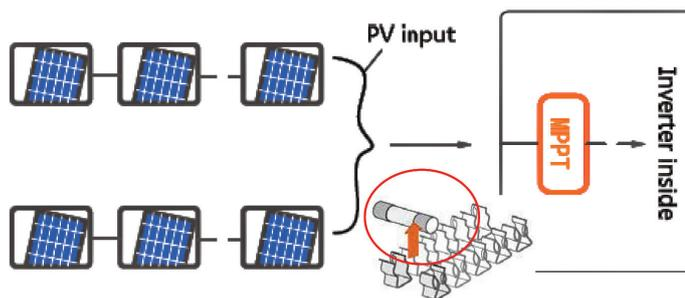
Adding DC fusing to each string is a costly and time-consuming addition to a design that can be avoided by limiting the number of strings per MPPT to two.
