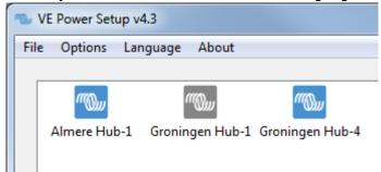
5. After selecting the site, VE Power Setup will establish communication to the selected site. Once established, it will perform a remote scan, to find all products connected to the Color Control. Now select the product you want to configure:
