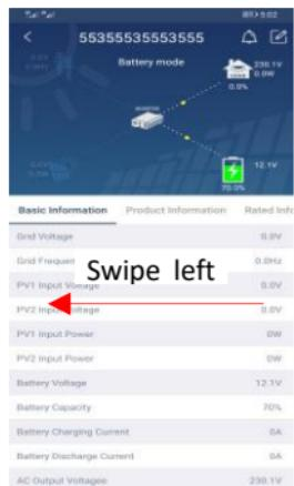
**【Basic Information】** displays basic information of the inverter, including AC voltage, AC frequency, PV input voltage, Battery voltage, Battery capacity, Charging current, Discharging current, Output voltage, Output frequency, Output apparent power, Output active power and Load percent. Please slide up to see more basic information.
