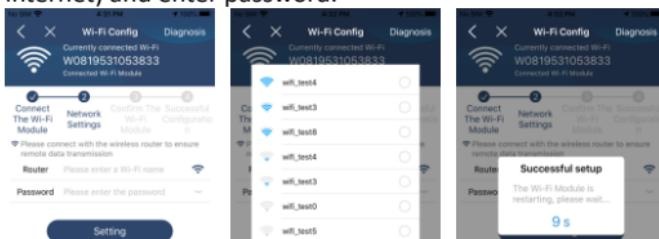
**Step 4:** Tap “Confirm” to complete the Wi-Fi configuration between the Wi-Fi Smart Card and the Internet.
