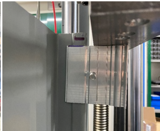
Figure 4 locking effects at the end of the shear tests
