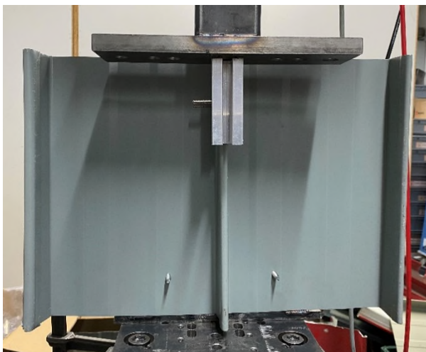
Figure 3 Test set-up for the shear tests
