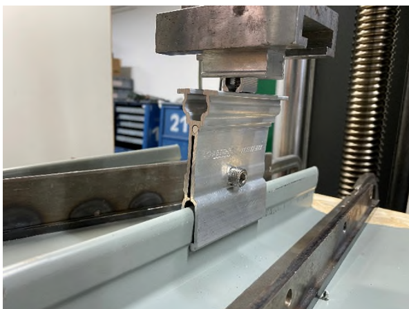
Figure 6 Test set-up for the tension tests
