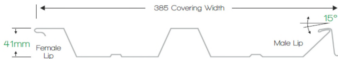
Fig. 1 schematic display of the profile cross section
