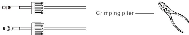
3. Insert the contact pin into the connector housing until it locks into place. Then screw the cap nut onto the connector housing. Torque to 2.5-3 N.m.
