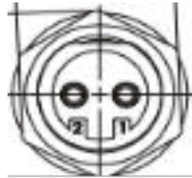
The following table presents the definition of the high-voltage control box interface PCS, IN, and OUT connection pins. All use the same pin number sequence shown in the next image:
