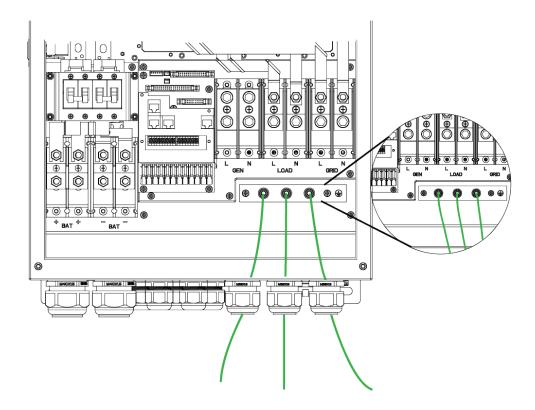
All neutrals can be linked together to maintain the neutral bond. When Neural Earth bond is required for 'Off-grid' operation, then it has to be removed on 'Grid-Tied' operation.
