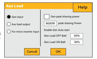
**Peak Shaving:** This is a technique used to reduce electrical power consumption during periods of maximum demand on the utility grid. This enables the user to save substantial amounts of money due to the expensive peak power charges.
