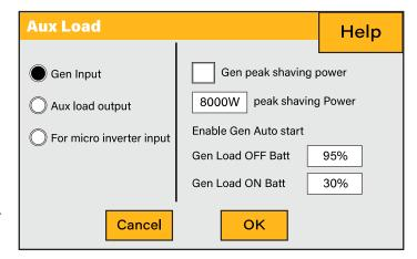
A nice feature of this page is that when the batteries are full and the inverter is still producing power from the solar PV or turbine, it is possible to direct the power generated to another load such as a water heater.
