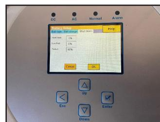
Figure 3: Battery Shut Down settings
