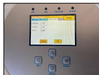
Figure 3: Battery Shut Down settings
