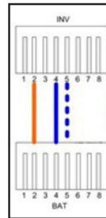
Figure 7: Pinout configurations for old Pylontech batteries
