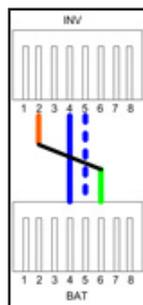
Figure 6: Pinout configurations for new Pylontech batteries
