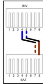
Figure 5: Sunsynk and Freedom Won BMS cable pinouts
