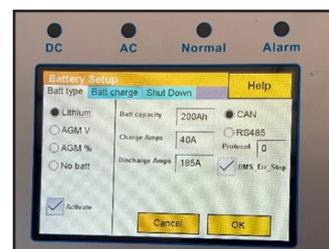
Figure 4: Battery type settings
