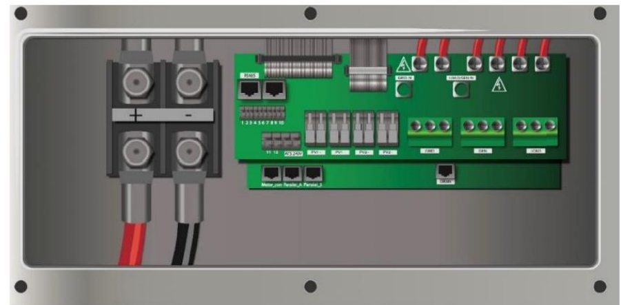
Battery connection of the 8kW model
