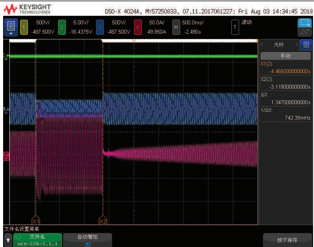
3.1.1(Channel 2: signal, channel 1: L2; channel 3: L1; channel 4: I1)
