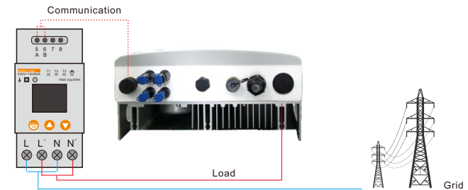
▲ Figure 4.23 Meter in Grid
