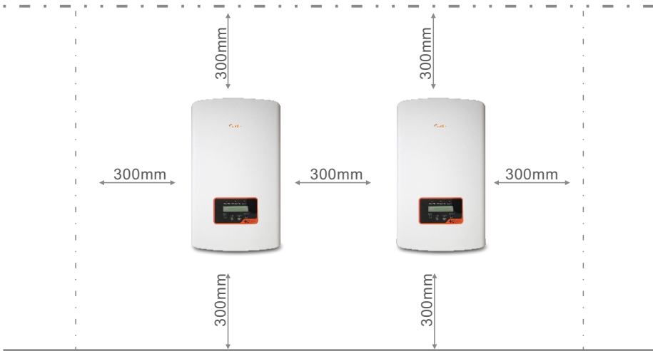
▲ Figure 4.2 Inverter Mounting clearance
