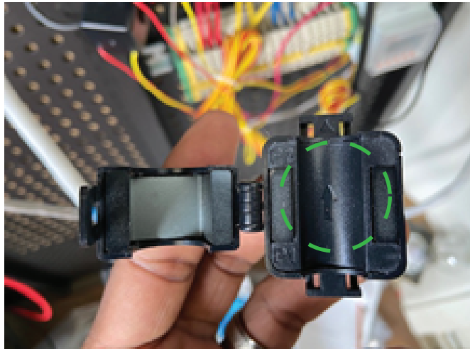
Figure 5: CT directional arrow
