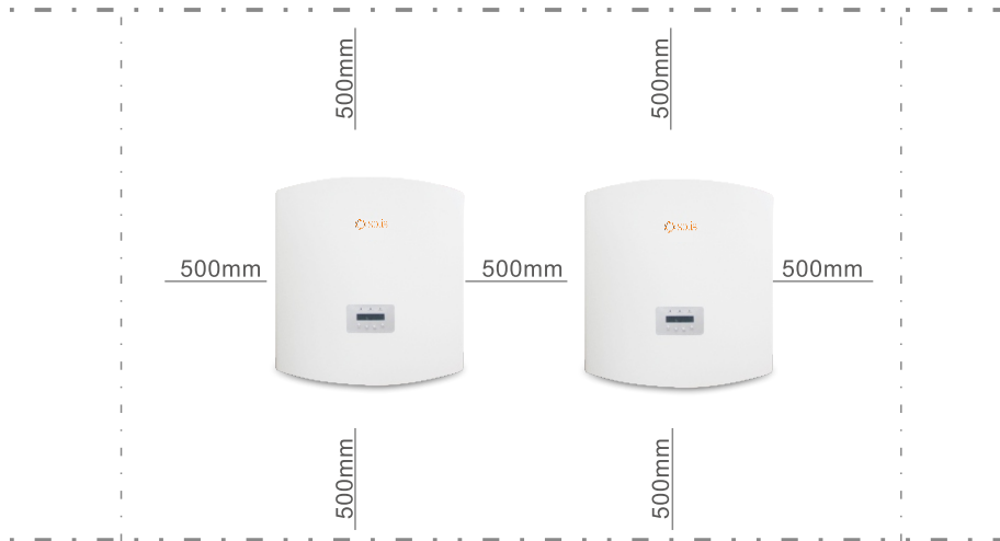
▲ Figure 5.2 Inverter mounting clearance
