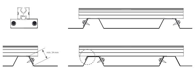
The mounting surface at the trapezoidal sheet must be at least 34mm high!
