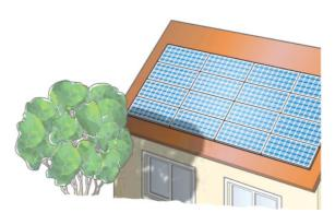
The difference between both heights and the distance to the shading object is used to calculate the elevation angle of the object. Now it is possible to add elevation and orientation of the object to the sun path, which provides the initial information on how often the object will shade the specific area and whether a detailed shading analysis might be necessary.
