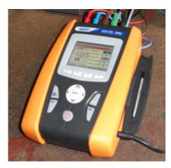
Direct Measurements: Current, Characteristic Curves, Power
