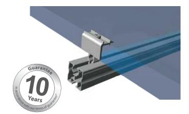
The Schletter module clamp range Rapid<sup>16</sup> provides a lot of advantages, such as better warehousing due to the minimised number of design variants and the grounding pin integrated in each module clamp. The Rapid<sup>16</sup> clamps are compatible with all Schletter module-bearing rails with 8 mm click channel, designed for module frames of 30 - 50 mm height.
