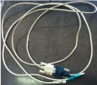
For US2000/US3000/Phantom-S/UP2500, the RS232 cable type is RJ11 – DB9 – USB:
