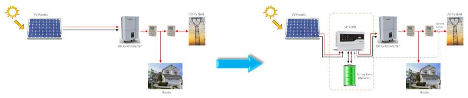
**PV Installation without Battery**
