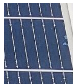
P5 cells showing visible border grains.
