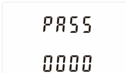
Setting up is password-protected so you must enter the correct password (default '1000') before processing. If an incorrect password is entered, the display will show: Err
