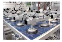
Example of a module loading test with vacuum suction (TÜV Rheinland)
