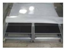
Example of a module loading test with water bag (Schletter) (Preparation of the test set-up)
