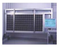
Example of a module loading test in an overpressure/underpressure test set-up (VDE)
