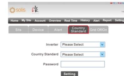
There are two remote setting functions of 'Grid Off/On', 'Country Standard', under the 'Setting' choice.
