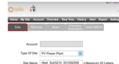
There are four remote setting functions of 'Grid Off/On', 'Country Standard', 'Controller' under the 'Setting' choice.
