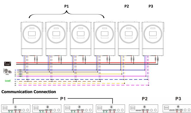
Three inverters in one phase, two inverters in second phase and one inverter for the third phase:
