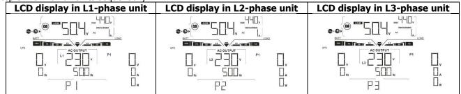
Step 4: Switch on all AC breakers of Line wires in AC input. If AC connection is detected and three phases are
