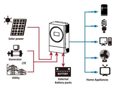
Figure 1 Basic hybrid PV System Overview
