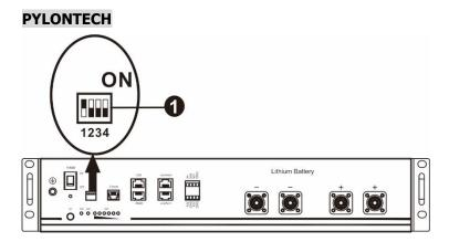
①Dip Switch: There are 4 Dip Switches that sets different baud rate and battery group address. If switch
