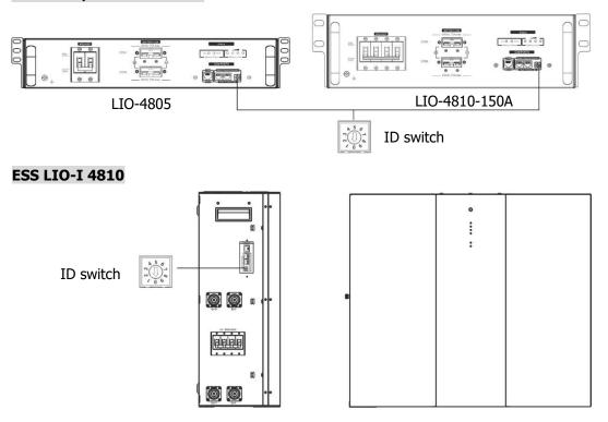
ID Switch indicates the unique ID code for each battery module. It's required to assign a unique ID to each battery module for normal operation. We can set up the ID code for each battery module by rotating the PIN number on the ID switch. From number 0 to 9, the number can be random; no particular order. Maximum 10 battery modules can be operated in parallel.
