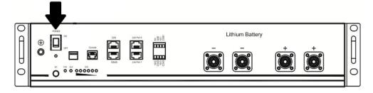
Step 3. Press more than three seconds to start Lithium battery, power output ready.
