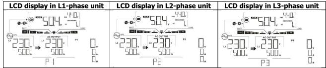
Step 5: If there is no more fault alarm, the system to support 3-phase equipment is completely installed.
