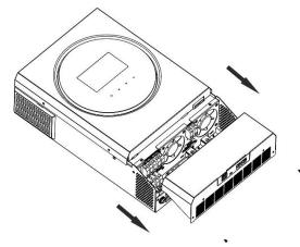
**Step 2:** Remove two screws as below chart and remove 2-pin and 14-pin cables. Take out the board under the communication board.
