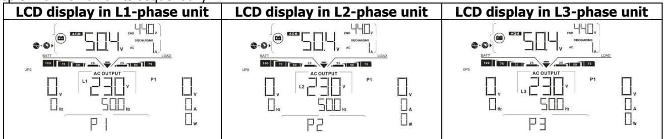
Step 4: Switch on all AC breakers of Line wires in AC input. If AC connection is detected and three phases are matched with unit setting, they will work normally. Otherwise, the AC icon
