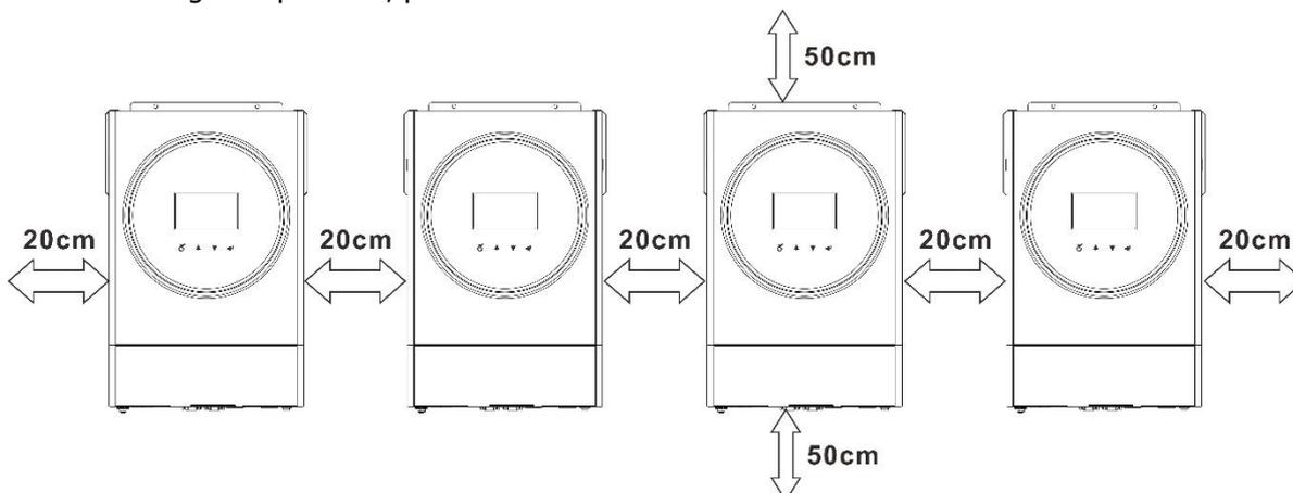
**NOTE:** For proper air circulation to dissipate heat, allow a clearance of approx. 20 cm to the side and approx. 50 cm above and below the unit. Be sure to install each unit in the same level.
