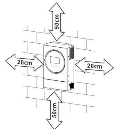
**⚠ SUITABLE FOR MOUNTING ON CONCRETE OR OTHER NON-COMBUSTIBLE SURFACE ONLY.**
