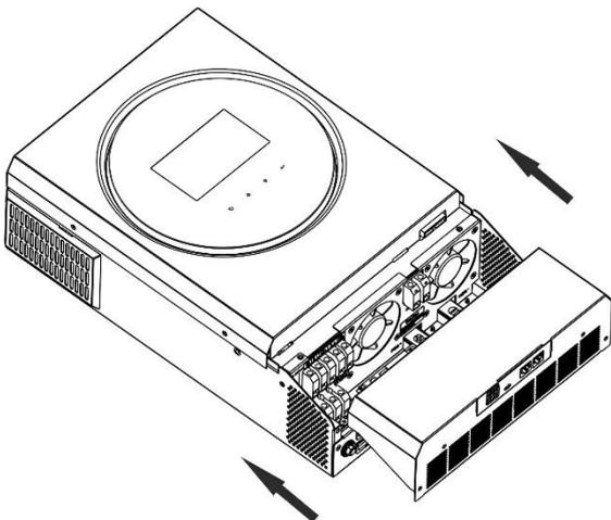
**Step 8:** Put wire cover back to the unit. Now the inverter is providing parallel operation function.
