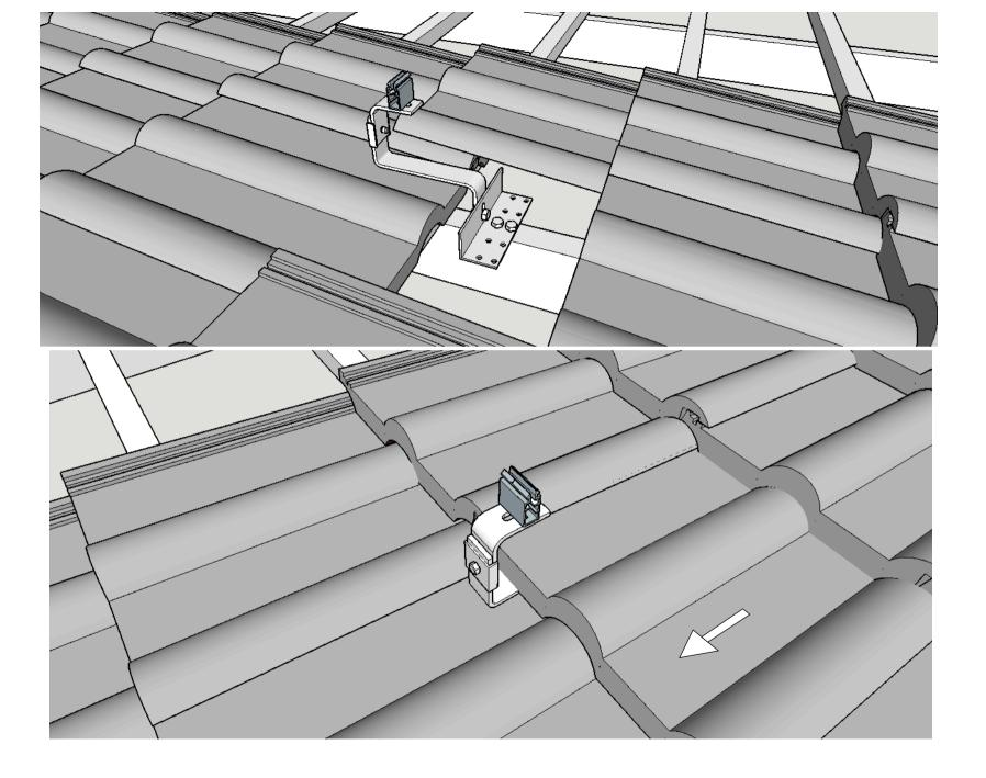
After bolts are fastened slide roof tile back over Tile Bracket as shown
