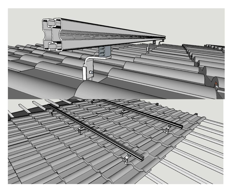
After all tiles have been moved back into position, clip the aluminium rail onto the exposed push-clip, an audible click must be heard. Ensure aluminium rails are evenly spaced over roof hooks. Tighten bolt under pushclip with 13mm spanner.
