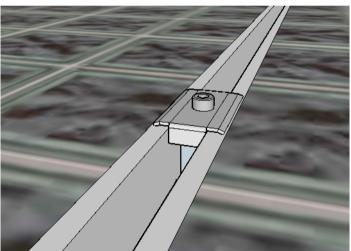
Install the second panel by sliding the solar panel under the middle clamp, repeat end clamp procedure.
