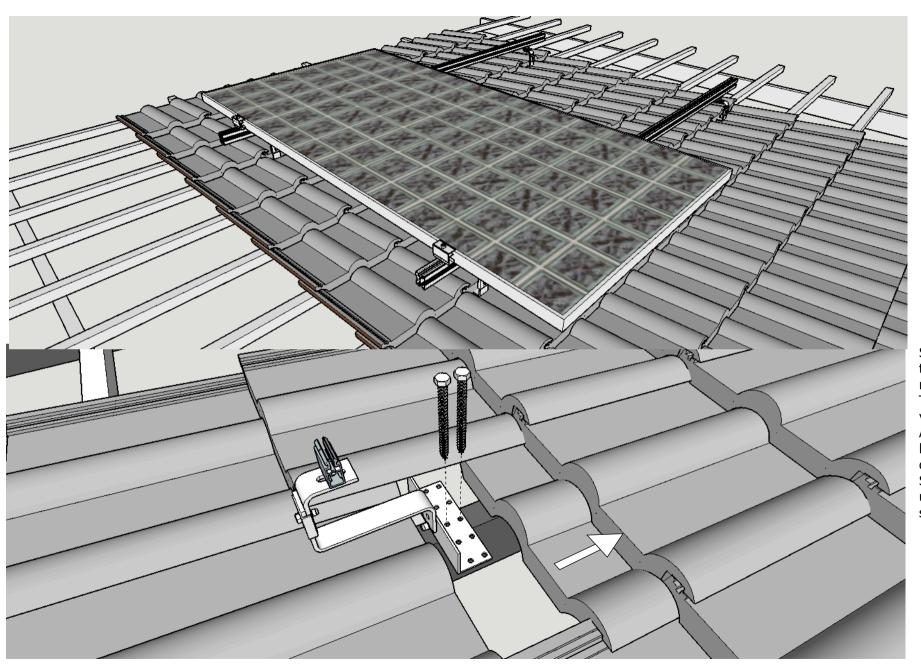
Solar panel end clamp position will vary with different size panels and manufacturers. Check solar panel data sheet for these measurements.
