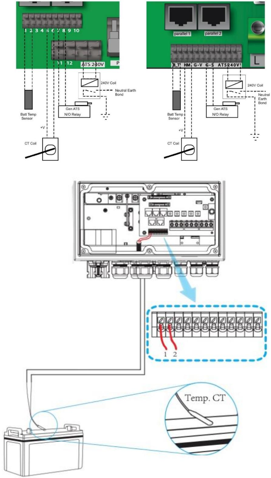
Without a remote temperature sensor, lead-acid batteries may undercharge or overcharge depending on the ambient temperature of the installation environment. This may result in a fire hazard.
