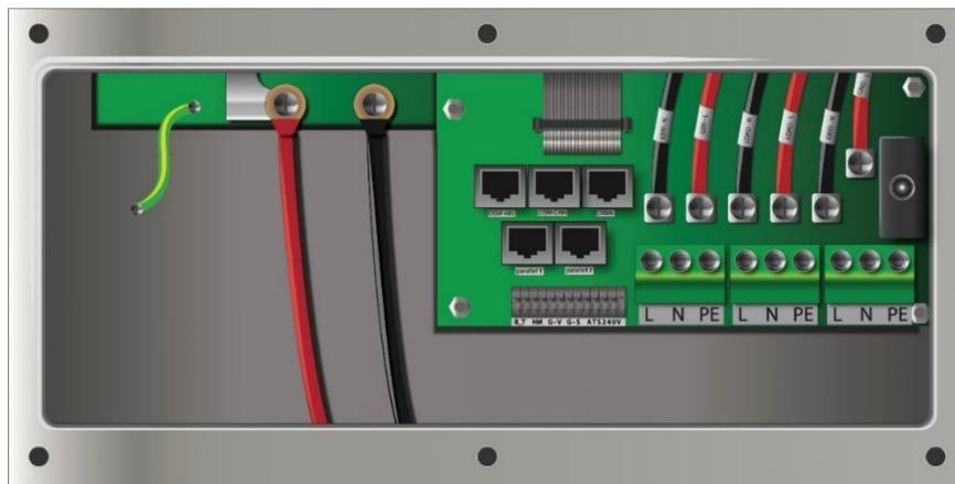
■ **Battery connection of the 8kW model**
