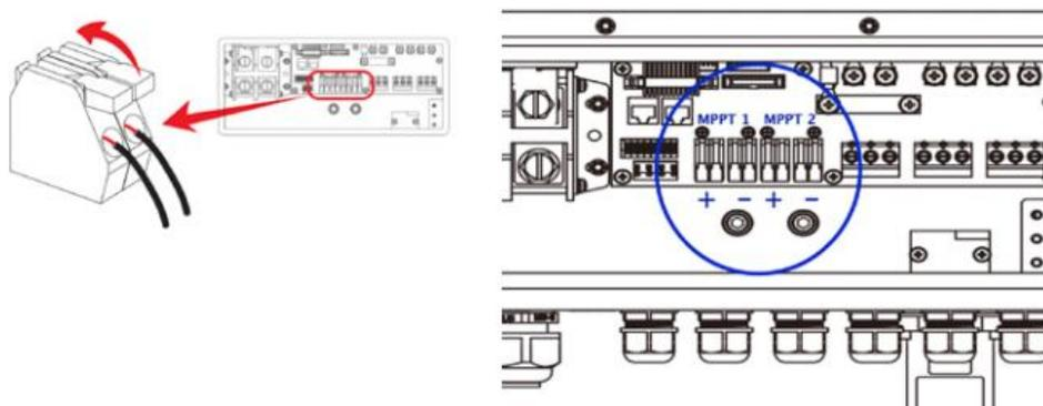
**5.5 KW PV panels are connected via the MC4 connectors located at the bottom of the inverter**
