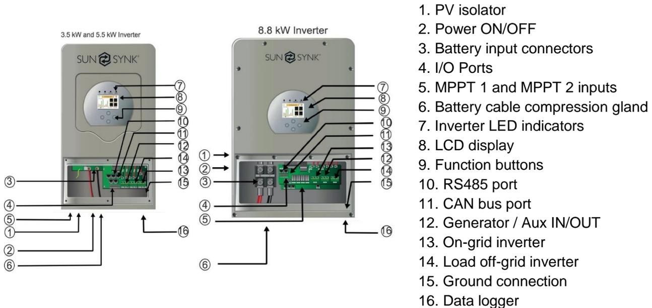
The Sunsynk Hybrid Parity Inverter is a highly efficient power management tool that allows the user to hit those 'parity' targets by managing power flow from multiple sources such as solar, main electrical grids, and generator, and then effectively storing and releasing electric power as the utilities require.
