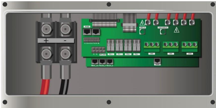
For safe operation and compliance, an individual DC overcurrent protector or disconnection device is required for the connection of the battery and the inverter. It is recommended to utilize a suitable fuse and DC isolator (see next page). In some applications, switching devices may not be required but overcurrent protectors are still required.
