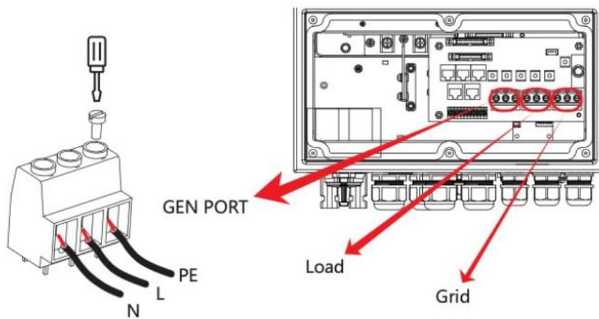
Check that AC power source is isolated before attempting to wire it to the inverter. Insert AC output wires according to polarities indicated on the terminal block and tighten terminal. Be sure to connect corresponding N wires and PE wires to related terminals and ensure the wires are securely connected.
