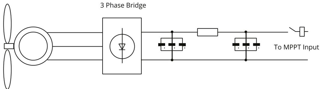
**Dump Load:** When the battery (battery bank) is fully charged and the water turbine/wind turbine/solar module is still generating power, a dump load will provide the electricity a path to flow. This can be done using a switch on by the smart load option or utilizing a wind turbine controller with a built-in dump load. Also, the hot water tank controlled via smart load can act as a good dump load, but in very windy conditions it may be necessary to shunt the output.
