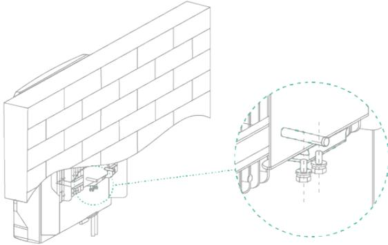
6. **Remove the bottom cover.** Remove the 2 screws on the bottom of the inverter with the Allen key. Pull down the bottom cover and push the grommet out of the way.
