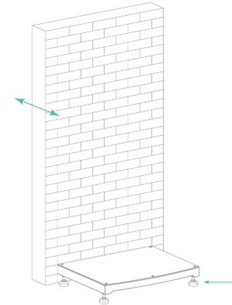
2. Stack the battery modules on the base making sure they are flush to the wall. Adjust the feet to make sure they are flush to the wall and level left and right. Once all of the battery packs are in place use the template to determine the location of the wall bolts. Ensure the template is level and completely flush to the wall.
