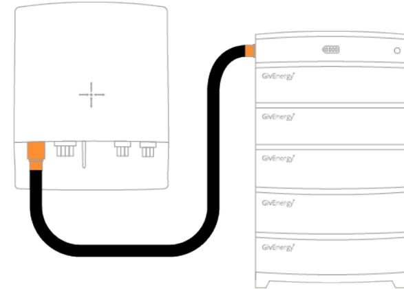
2. Make sure there is one cable (under local legislation, 6mm<sup>2</sup> earth cable suggested) running from one of the earthing points on the bottom of the inverter to the earthing point on the stackable battery.
