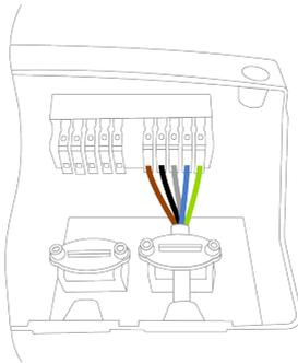
8. You must install a separate AC circuit-breaker per inverter in order to ensure that it is adequately protected and can be safely disconnected under load. Please follow local legislation.
