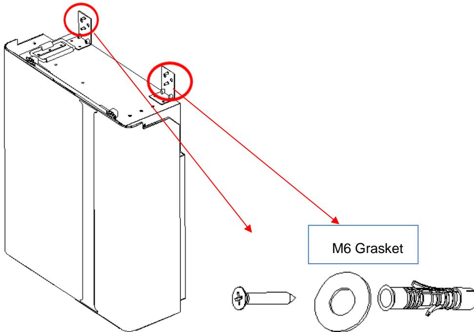
Step 5: Insert the expansion tube into the drilled hole. Pass the expansion screw through the gasket and lock with a screwdriver.
