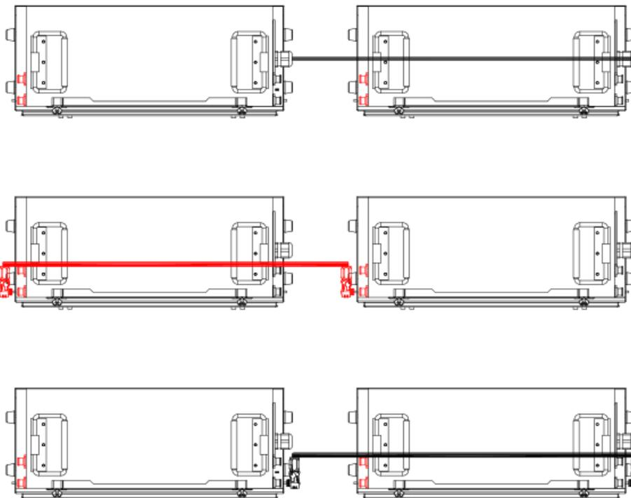
Step 9: Please connect the positive pole of one battery to another with red power cables, connect the negative pole of one battery to another with black power cables and connect one battery com port to another battery com port as the above figure shows.
