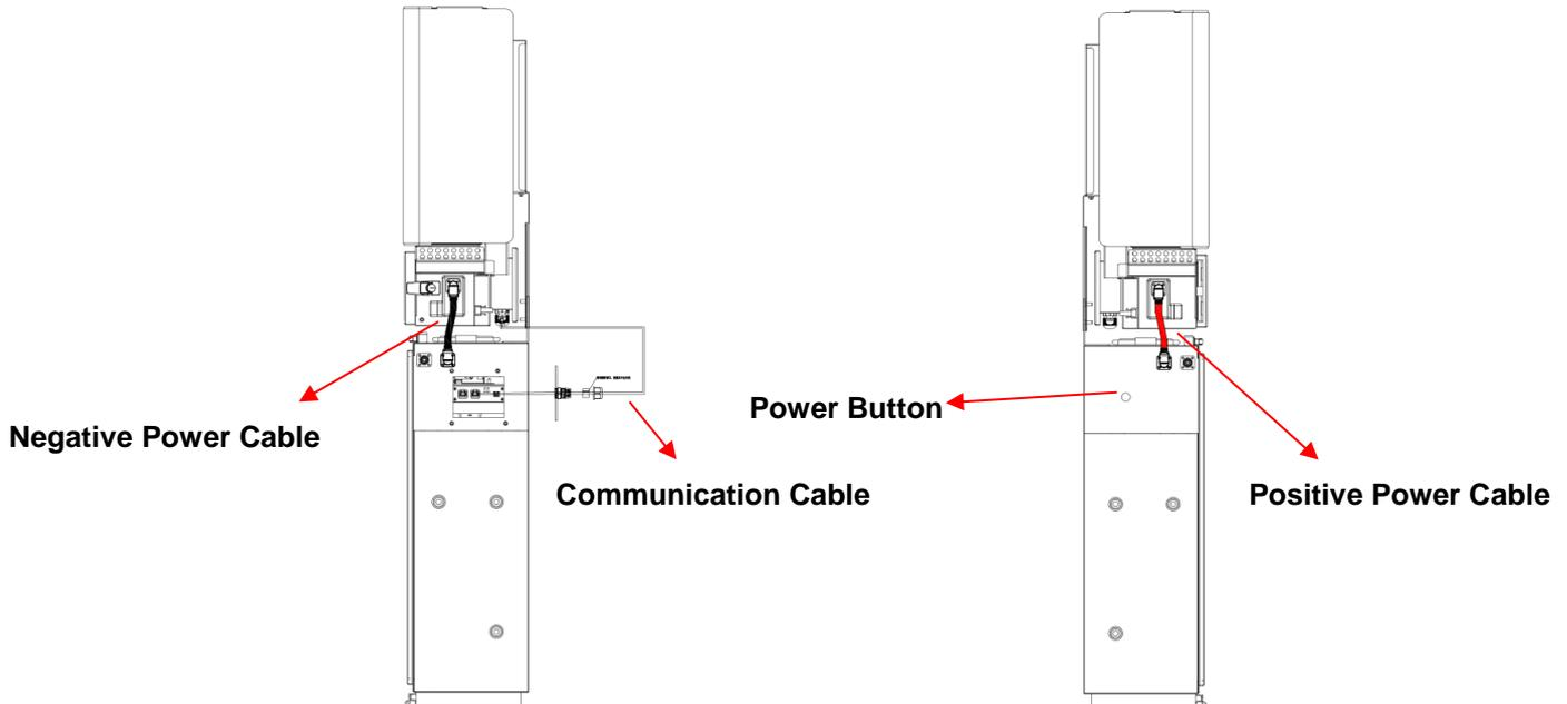
Step 6: Install the inverter above the battery, please refer to the SMILE5 Installation Manual.
