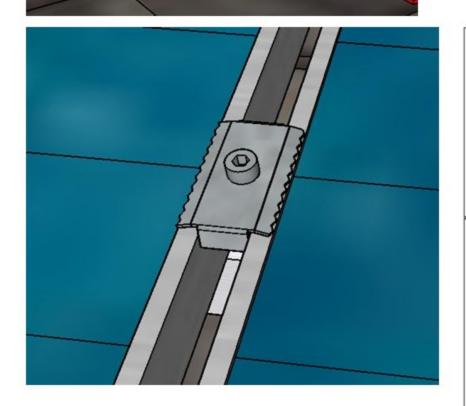
When installing the middle clamp, clip the push-clip into the aluminium rail, make sure you hear the audible click. Move the middle clamp so the bent spacer is flush against the Solar panel.
