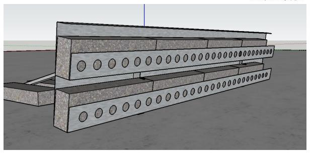
INSTALL THE BALLASTS. PLACE TWO BALLAST IN THE FRONT OF THE A FRAME, TWO PER BALLAST HOLDER.
