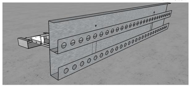
FASTEN THE REAR BALLAST HOLDERS TO THE REAR OF THE A-FRAME USING THE TEKSCREWS PROVIDED. TWO ROWS OF BALLAST HOLDERS MUST BE INSTALLED ONTO THE REAR OF THE A FRAME
