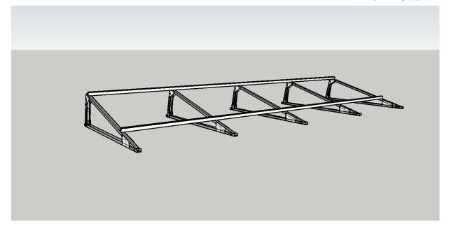
SPACE YOUR A FRAMES AND FASTEN THE RAIL ONTO THE TOP OF THE A FRAME USING THE BOLT, NUT, WASHER SUPPLIED.
