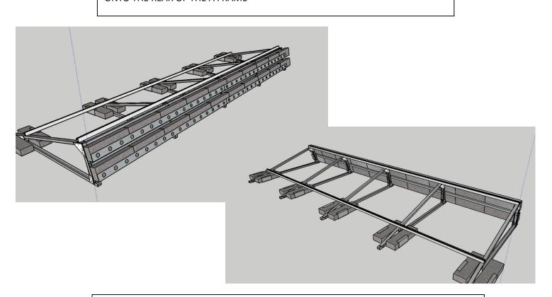
INSTALL THE BALLASTS. PLACE TWO BALLAST IN THE FRONT OF THE A FRAME, ONE PER BALLAST HOLDER.
