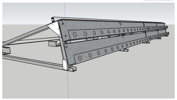
FASTEN THE REAR BALLAST HOLDERS TO THE REAR OF THE A FRAME USING THE TEKSCREWS PROVIDED. TWO ROWS OF BALLAST HOLDERS MUST BE INSTALLED ONTO THE REAR OF THE A FRAME
