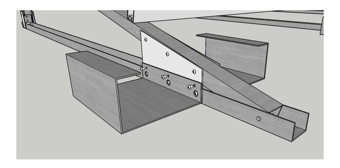
USING THE POPRIVETS SUPPLIED. FASTEN THE FRONT BALLAST HOLDER TO THE FRONT OF THE AFRAME. POPRIVET USING THE DESIGNATED HOLES
