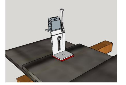
Fasten the Slate/Harvey bracket in place by sliding the red silicone seal between the bracket and tile. Fasten with screw provided.
