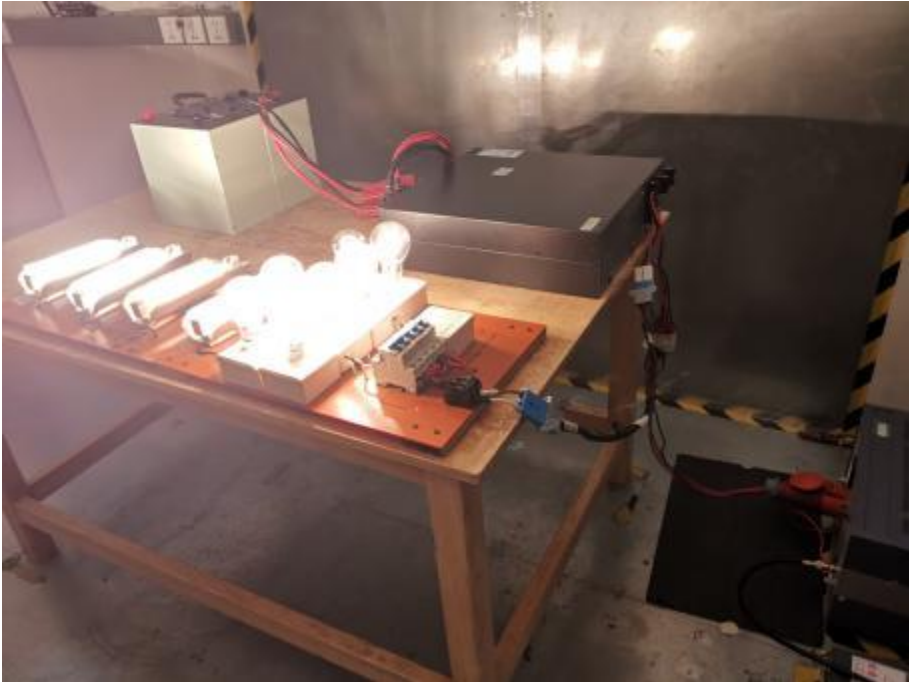
16.1 Photo of Conducted Emission Measurement
