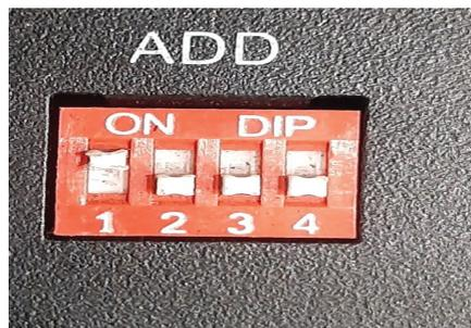
Figure 1: BMS module dip switches
