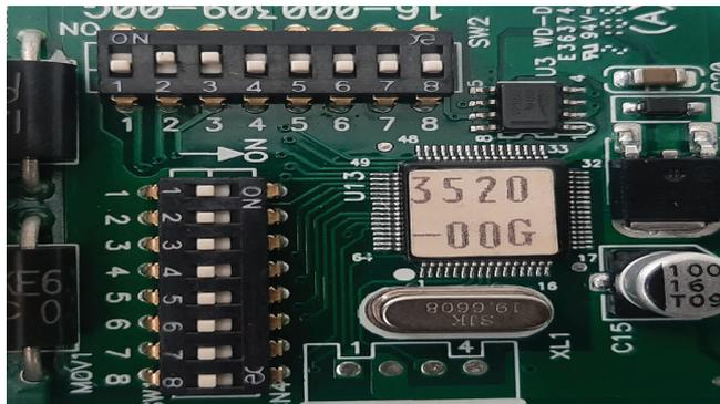
Figure 2: BMS card dip switches
