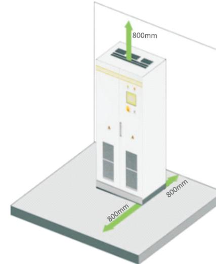
In front of the installation place of inverter, a space of 0.8m or more shall be ensured, the back 0.8m or more, the top 0.8m or more to ensure easy installation, cooling and maintenance.
