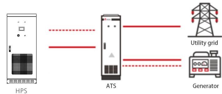
3. There are three circuit breakers in ATS. The middle circuit breaker is connected to the power grid switch (AC input) of HPS. The other two are grid switch (grid) and generator (Gen) switch. Pay attention to the printing on cabinet. It is not allowed to connect incorrectly, neither is it for the three phase sequence, otherwise the system cannot operate normally.
