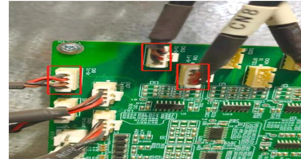
3. There are also corresponding number on the sampling cables (CN8, CN9, CN10, Grid-A, Grid-B, Grid-C)
