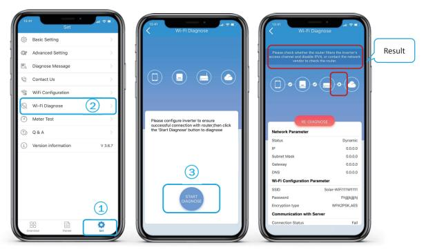
NOTE: Wi-Fi Diagnose is only available if PV Master is connecting to inverter Solar-WiFi signal directly.
