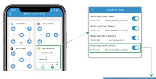
There are 4 editable different repeating logic, for each, you can set different date(s) and charge/discharge logics.
