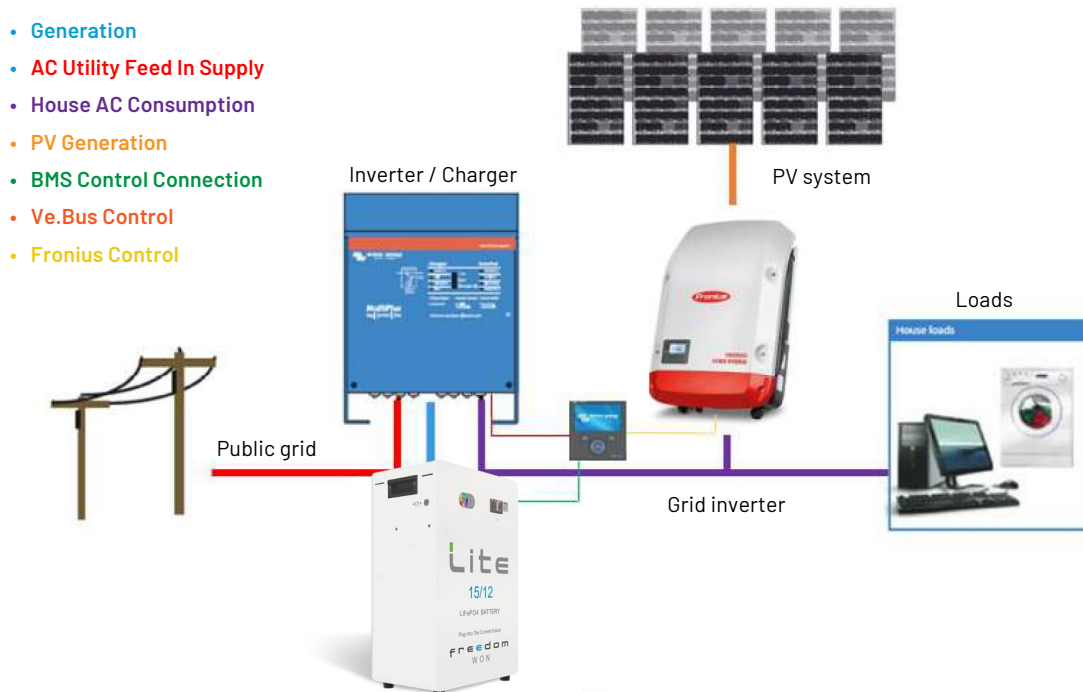
Figure 5.2 Installation Example using a Victron Battery Inverter and a Grid Tie Inverter with a LiTE Home 15/12.
