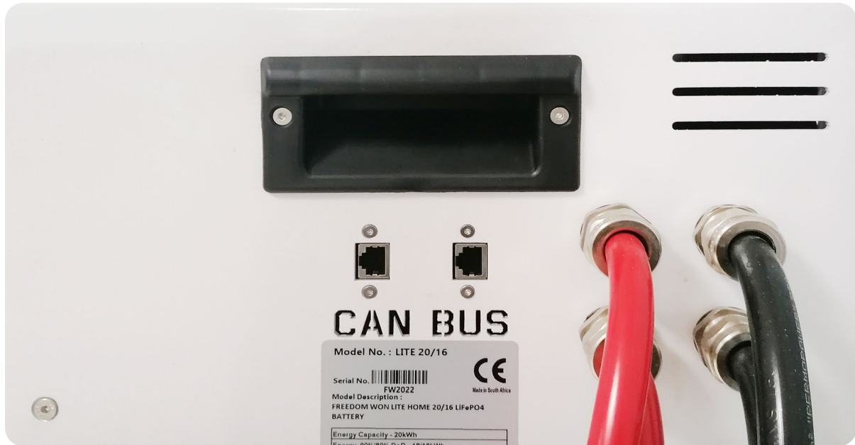
Figure 5.2 Picture Showing 2 x RJ45 Sockets for CAN Bus (DB15 Plug shown here for Analogue and Relay control is not available in new models)
