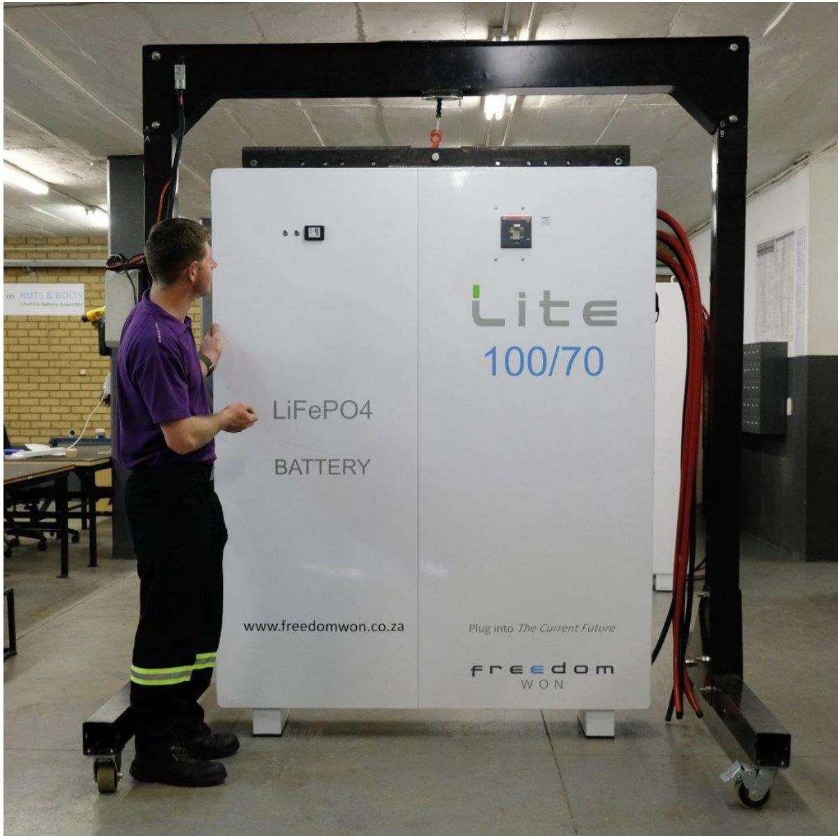
Fig 3.5 Site Assembled Gantry with Electric Winch
