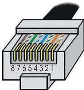
Fig 4.1 Pin Configuration for standard RJ45 plug
