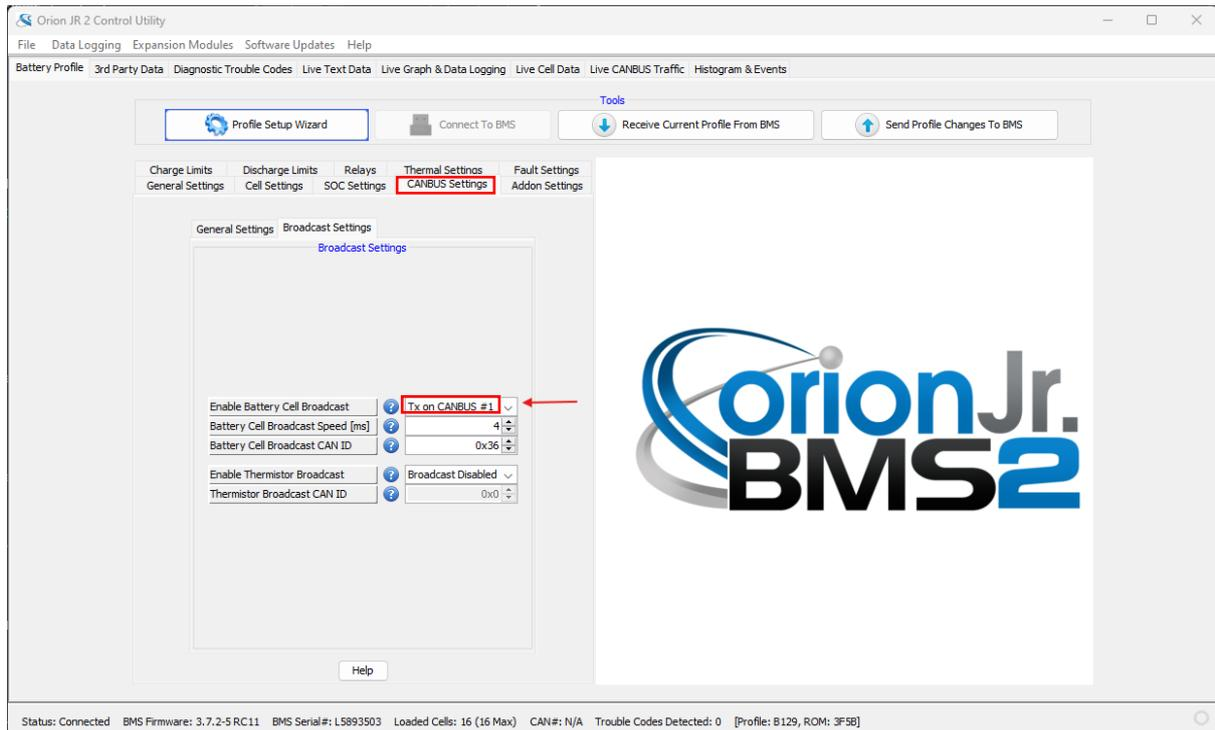
Figure 6: Enable Battery Cell Broadcast
