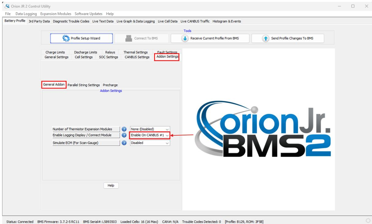
Figure 5: Enable Logging display on CANBUS #1
