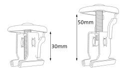
The integrated height adjustment fixes modules from 30mm to 50mm in height
