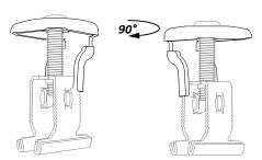
Change from end- to mid clamp function by a simple 90° head twist
