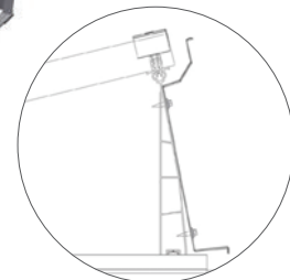
Simple alignment (e.g. southward), incline: about 13° with Windsafe sheets for ballast optimization
