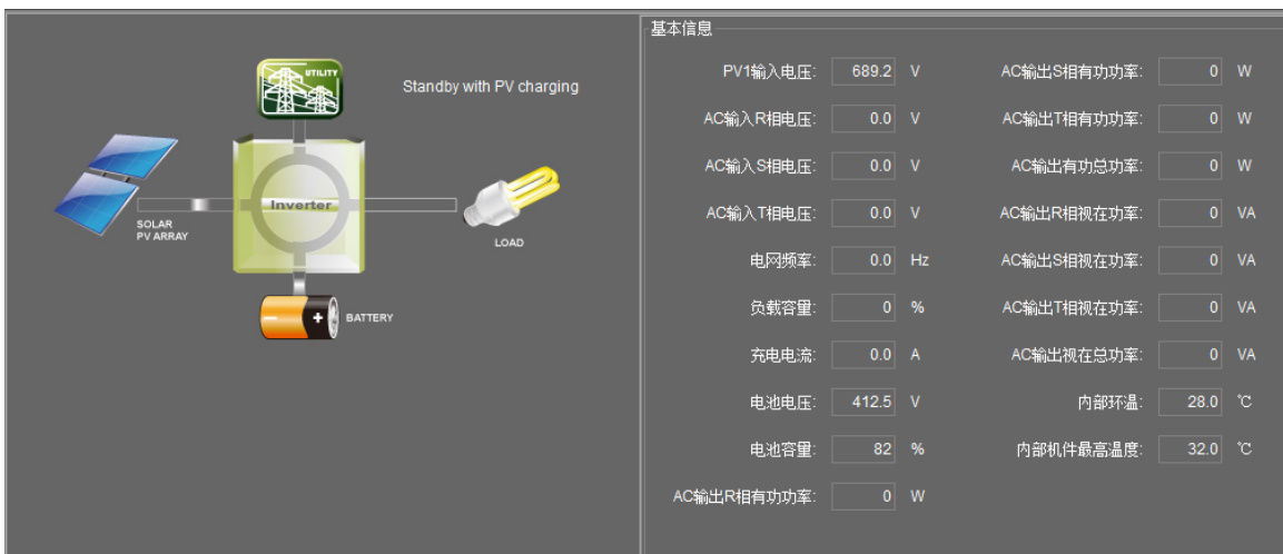
Fig3 in Standby with PV charging mode
