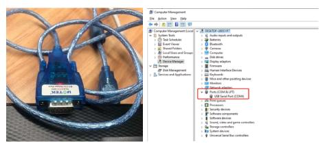
1.1.2. Then insert USB rs232 cable to the control board, and turn on the battery breaker supply the power for HPS, then running the DSPtool software.
