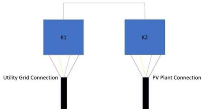
Recommended Cable Size: Main Cable - **70mm<sup>2</sup> x 4C**, Earth Conductor – **50mm<sup>2</sup> x 1C**
