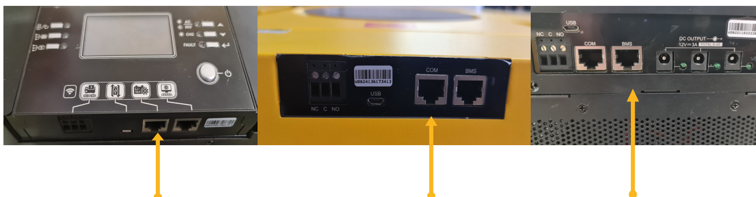
Figure 3: RS485 port of inverter
