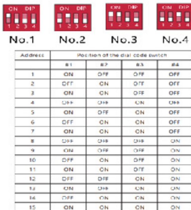
Figure 4: DIP switch configuration
