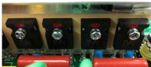
For VMIII-5000 ALL of the IGBTs are (IGBT ST/STGW60H65DFB 60A 650V N BULK TO-247)
