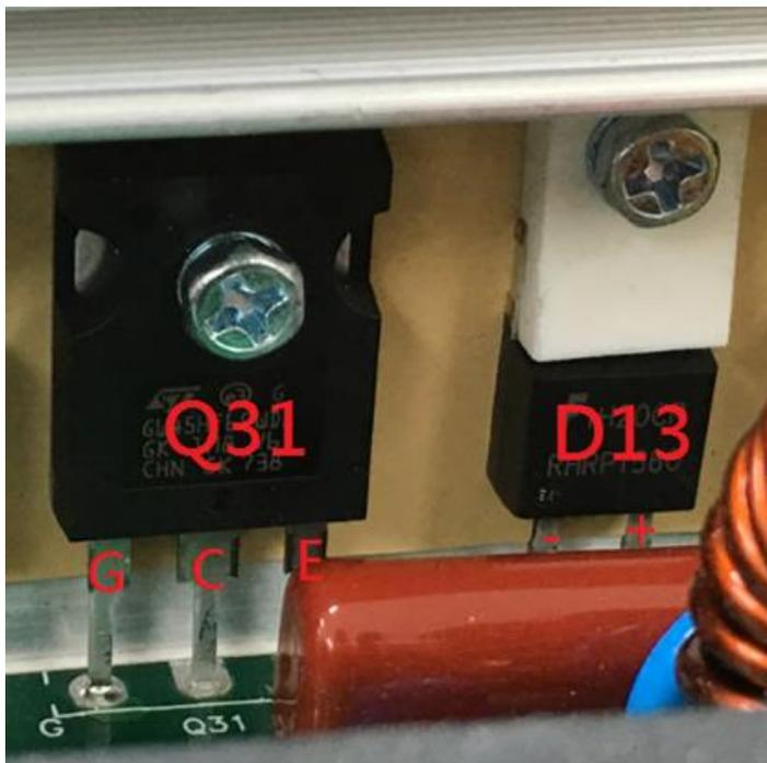
For VMIII-5000 the IGBTs Q31 is (IGBT ST/STGW60H65DFB 60A 650V N BULK TO-247)
