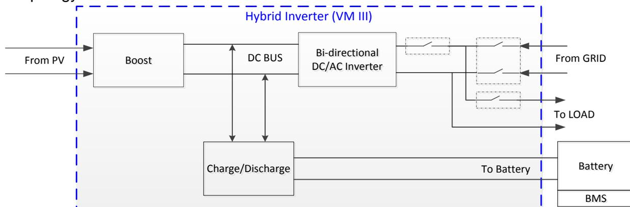
Compare with UPS or normal inverter, INVERTER combines a solar charger inside. Solar charger can be a supplement for battery when there is not grid. And with the solar charger, the inverter can have more working modes than UPS. For detail information please refer to our user manual.
