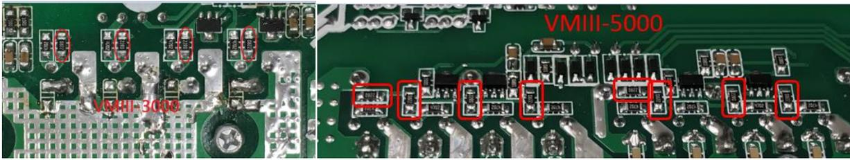
Use multimeter to measure each resistor, find the burnt resistors and replace them; don't need to replace them all.
