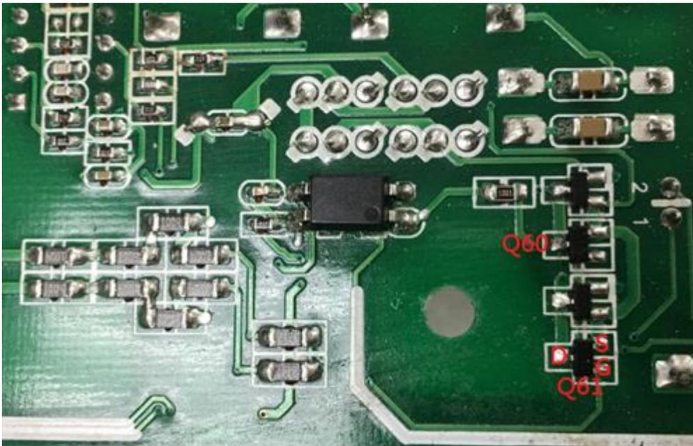
The Q60 and Q61 the MOSFET are (UT3404G 5.8A 30V NPN SOT-23 SMD)
