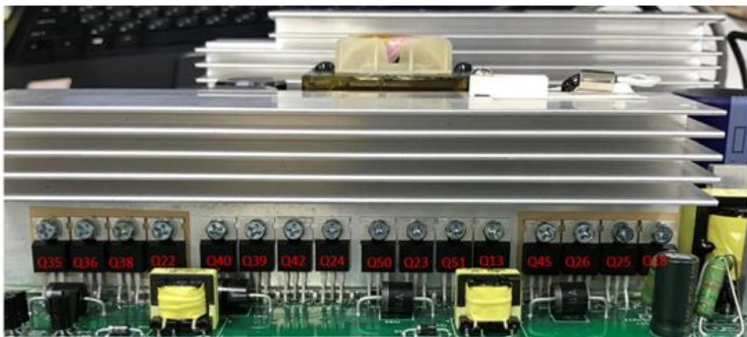
For VMIII-5000 ALL of the MOSFET are (MOSFET TOSHIBA/TK100E08N1 214A 80V N BULK TO-220)
