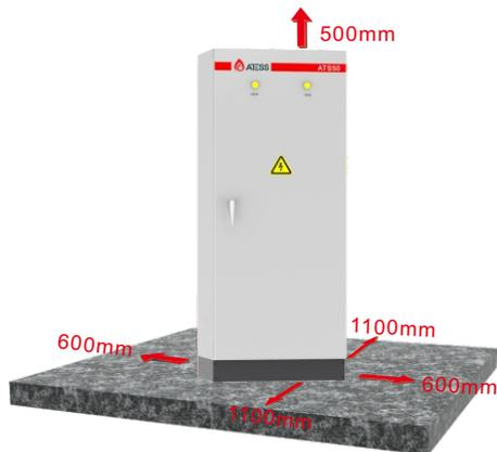
In front of the installation place of ATS, a space of 1.1m or more shall be ensured, the back 1.1m or more, the top 0.5m or more to ensure easy installation, cooling and maintenance.
