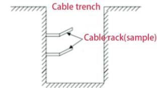
The cable trenches are often designed and constructed by the construction side based on relevant standards, with the equipment weight and dimensions required to be considered. Good electrical connection is needed between different cable trenches and GND terminals.
