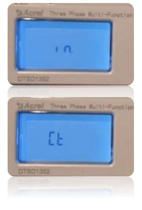
At this point is where we must indicate the ratio between the primary and secondary. For example, if we have a toroidal with a ratio of 150A - 5A, we must enter 30 as the ratio (150/5=30).
