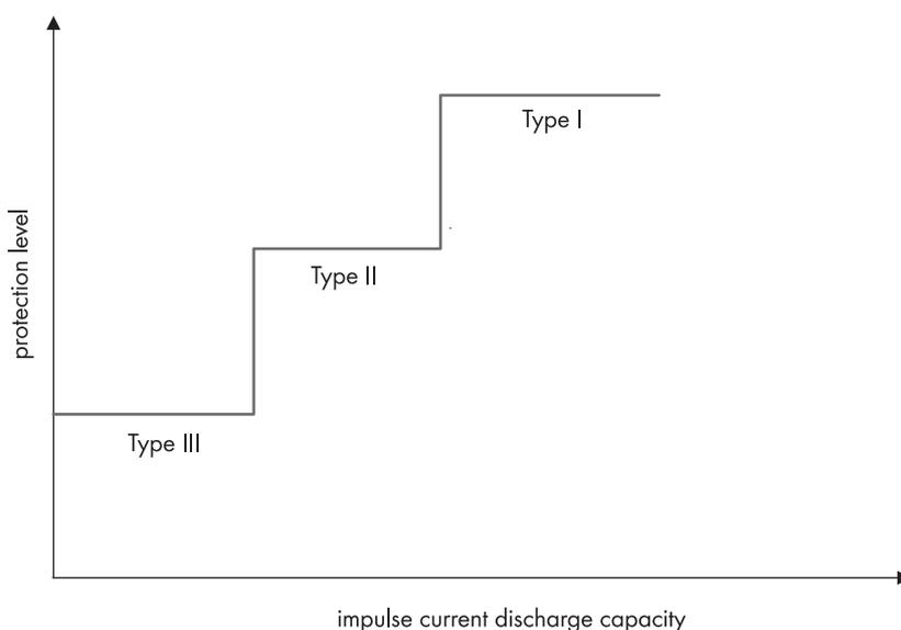
Fig. 2: Protection level of SPD with different values for admissible surge current resistance
