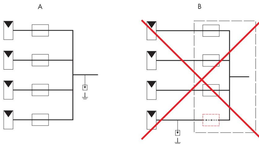
Fig. 5: Multiple strings with string fuses and a common SPD at the point of interconnection point (A), multiple strings with string fuses and an SPD connected to a string with tripped string fuse (B)
