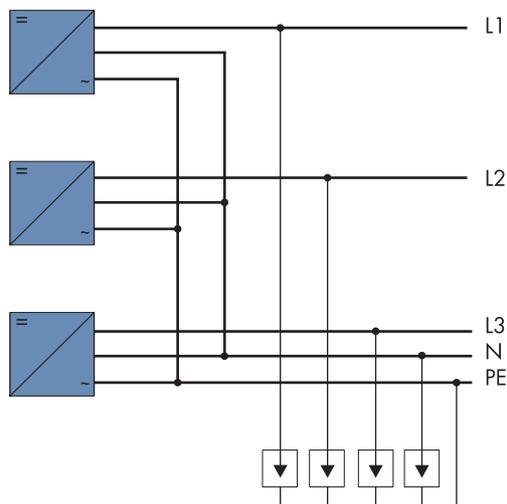
Fig. 4: AC-side connection of multiple inverters to a three-phase overvoltage protection device
