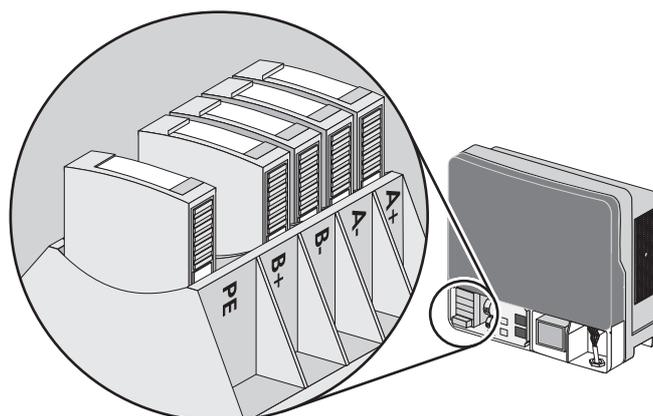
Fig. 7: Installation site of the SPDs with the STP XX000TL-10 device family as an example
