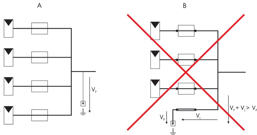
Fig. 6: SPD downstream of string fuses (A) and SPD connected to a string input where the string fuse has been replaced by a copper bolt (B)
