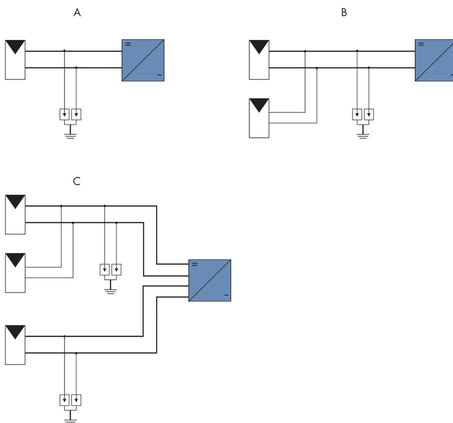
Fig. 3: A string connected to an inverter with one MPP tracker (A), multiple strings connected to an inverter with one MPP tracker (B), multiple strings connected to a multi-string inverter with multiple MPP trackers (C)
