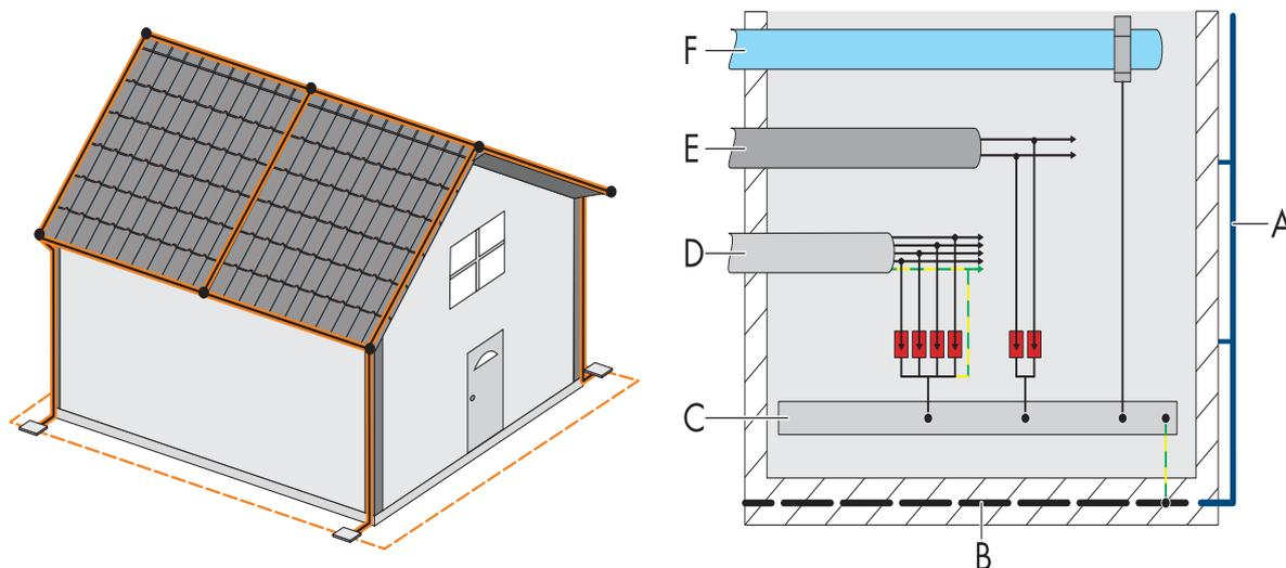
Fig. 1: External lightning protection (left) and internal lightning protection (right). Legend: A: external lightning protection (with connection to foundation ground electrode), B: foundation ground electrode, C: grounding busbar, D: grid connection, E: telephone connection, F: water pipe
